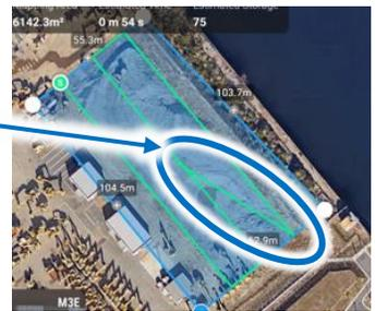
Maximum flight speed is not a problem. Higher speeds may cause the flight path to be rounded and the drone to shake more. If high accuracy is desired, the speed must be reduced.
