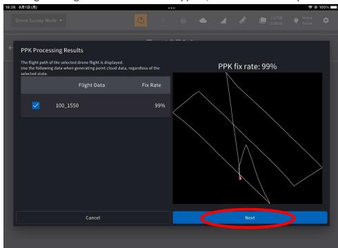
7. A dialog showing the PPK Fix rate will appear, check the rate and press "Next".
