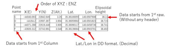
Unit of XYZ and Elipsoidal height are in feet.
