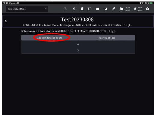
5. Tap "Install above reference point" . Enter the point name, pole height, and coordinates of the EdgeBox location, and tap "Add
