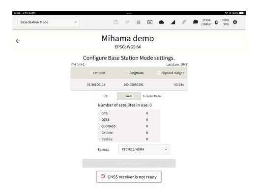
If the mobile station side (construction equipment, drone, GNSS rover) can receive compensation data from WIFI, compensation data via WIFI at the EDGE2 is available.
