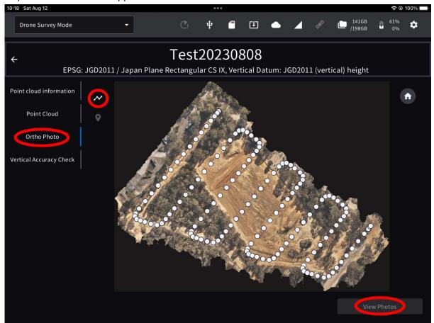
Displays the flight path of the drone. Tap  $\bigcirc$ , then tap the "View Photo" button to show the image taken at that point.
