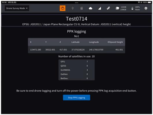
2. If GNSS reception deteriorates during the logging period, an error message may be displayed.
