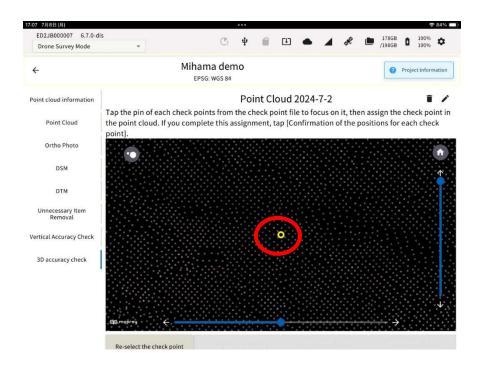
7. The position of the pink pin can also be fine-tuned with the cursor in the lower right corner. After placing it at the center of the verification point on the point cloud, tap "Confirmation of the positions for each check point" icon.
