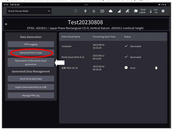
Tips Reservation of the point Cloud can automated processing from PPK to Upload-to-Dashboard without manual intervention.
