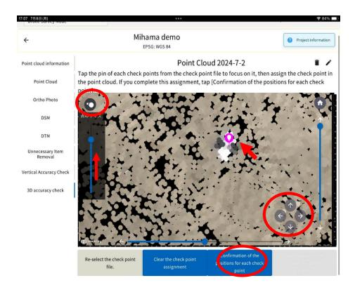
8. The pins of the validation points for which positions are specified turn light blue.
