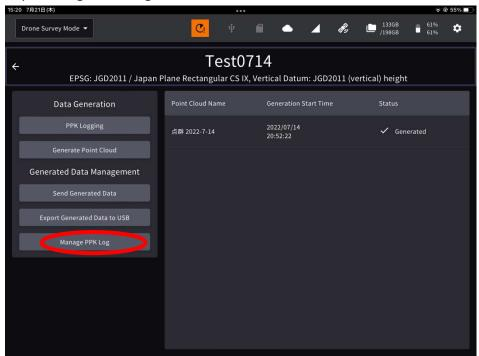
Displays the list of GNSS logs for the selected project.
