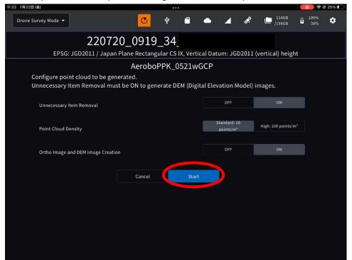
18. The point cloud viewer screen shows up and the point cloud generation process starts. During this process, it is possible to switch to another window and perform the other work. You can check the generated point cloud by selecting it from the list on the project top screen.
