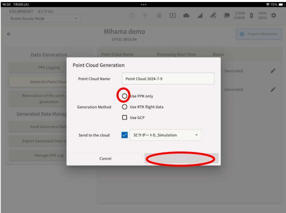
You can also improve the point cloud accuracy by using GCPs. Please see P.42. Using RTK flight data will be the same except the PPK data processing process.
