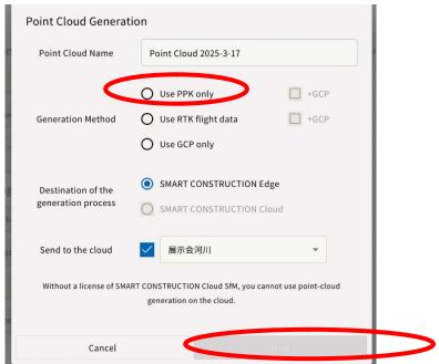
."If Edge 2 cannot be included in the drone photo, a GCP marker can be used to improve the accuracy of the point cloud. When Edge 2 is included in the drone photo, it serves as a GCP, allowing high accuracy with PPK-only processing.".
