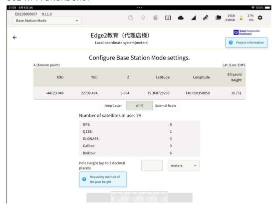
If the mobile station side (construction equipment, drone, GNSS rover) can receive compensation data from WIFI, compensation data via WIFI at the EDGE2 is available.
