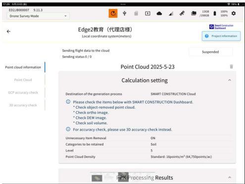
Once point cloud generation is complete, the point cloud will be displayed in the Edge2 application.
