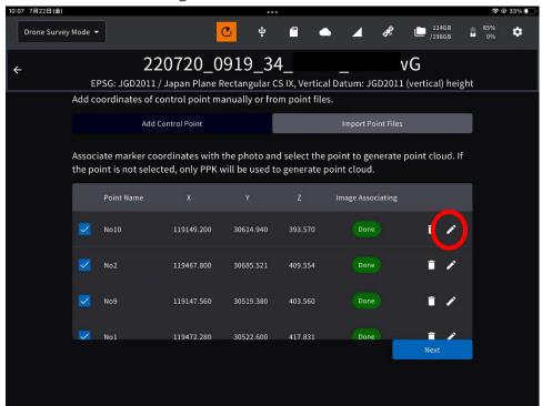
14. Tap the thumbnail of the image, align the center of the cross mark to the center of GCP in the image, and tap "OK"
