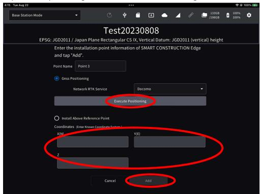
When the positioning was completed, coordinates are automatically entered to the fields.
