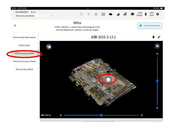
Select a point that you think is the center of the GCP and scroll down the screen to display the residual between the GCP center and the coordinates.
