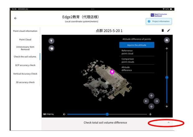
3. Select the point cloud for comparison and press "Calculate the soil Volume".
